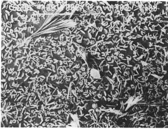
Fig. 10 SEM micrograph illustrating morphology of \text{CaCO}_3 crystals on SS-316 coupon exposed for 2 h to the scale forming solution in the test loop—magnification 200 \times
