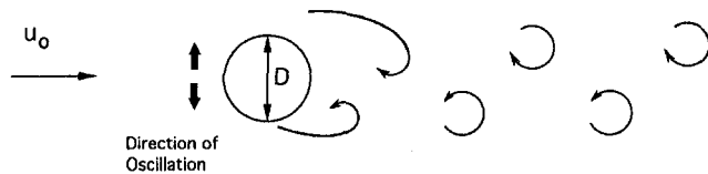
Fig. 1 A circular cylinder oscillating in a uniform stream
