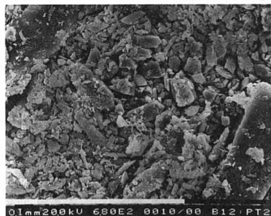
Fig. 5 Scanning electron microscope micrograph of calcium sulphate particles present in the solution once calcium sulphate deposits were formed on the heat transfer surface
